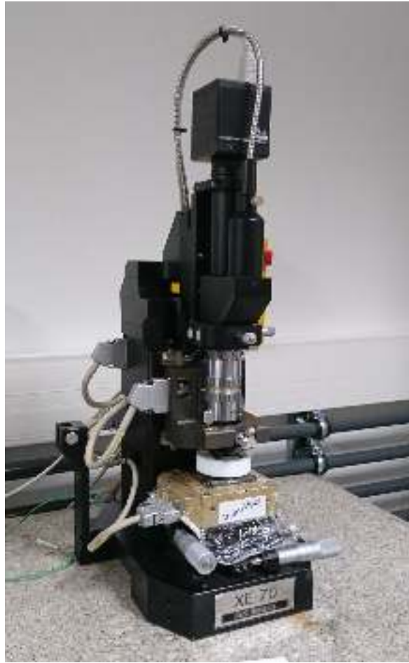
Figure II.2.5 – The XE-70 Park AFM instrument. A teflon sample cell is mounted on the instrument.
