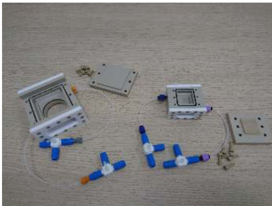
Figure II.2.15 – Developed solid/liquid cells suitable for XRR experiments in-house (smaller cell) and synchrotron (bigger cell) experiments.
