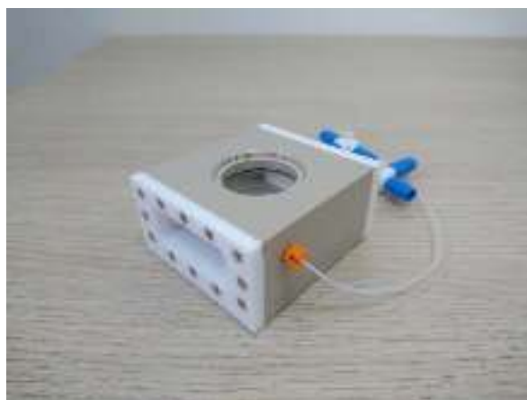
Figure II.2.13 – Solid/liquid cell for X-ray reflectometry experiments at the synchrotron.
