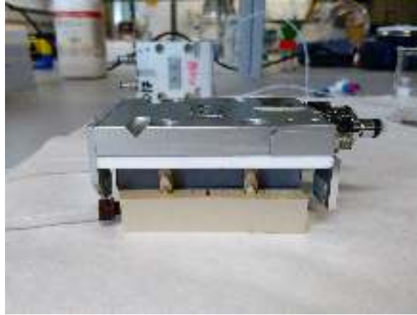
Figure II.2.24 – Solid/liquid cell used for the neutron reflectivity measurements.
