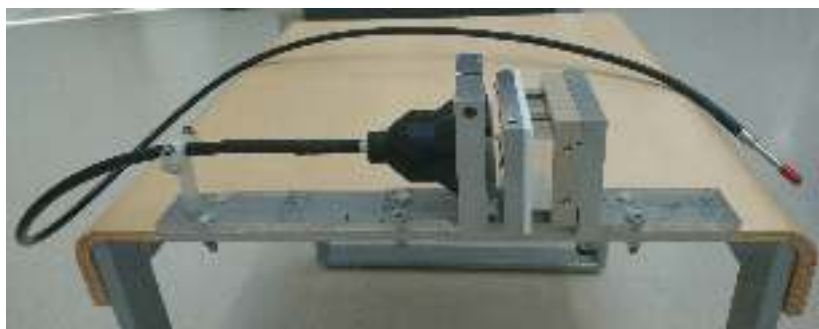
Figure II.2.10 – Setup for in-situ sample illumination during NR experiment.
