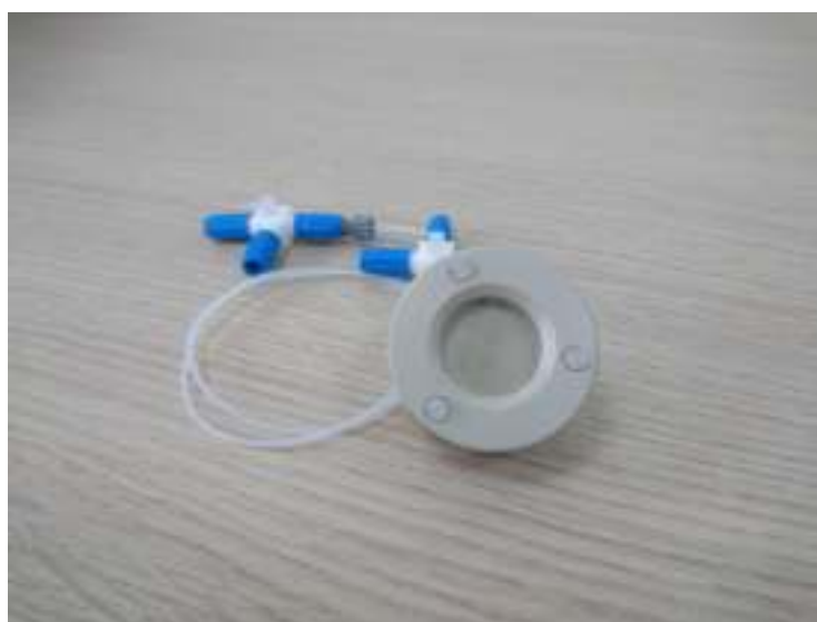
Figure II.2.12 – Solid/liquid cell for fluorescence microscopy experiments.
