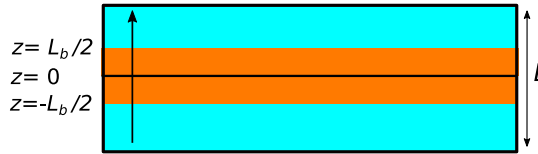
FIGURE 3.3 – Geometric parameterization of the system used in the present study, with L = L_b + L_w .
